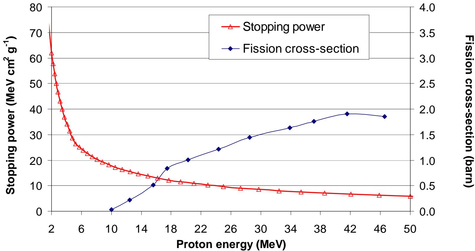
For lower power deposition in uranium keeping high fission rates:
